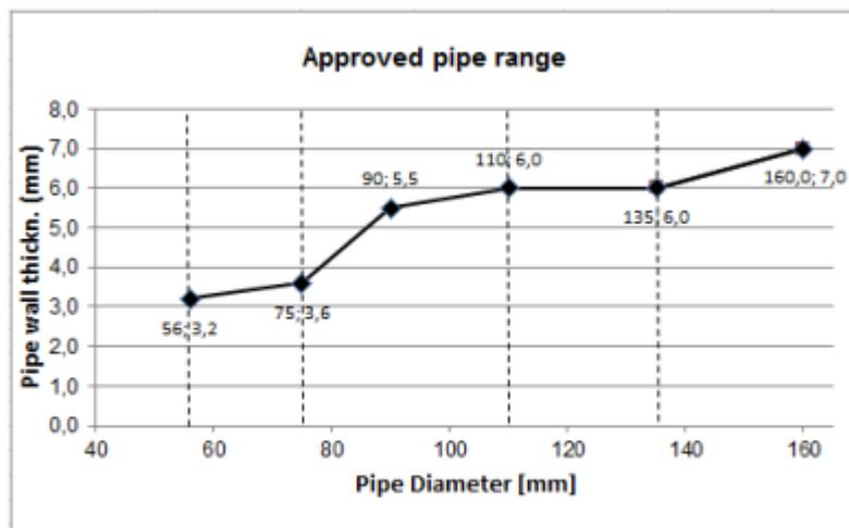
**2.2.3 PVC pipes acc. to EN 1452-2, EN 1329-1, EN 1453-1**
