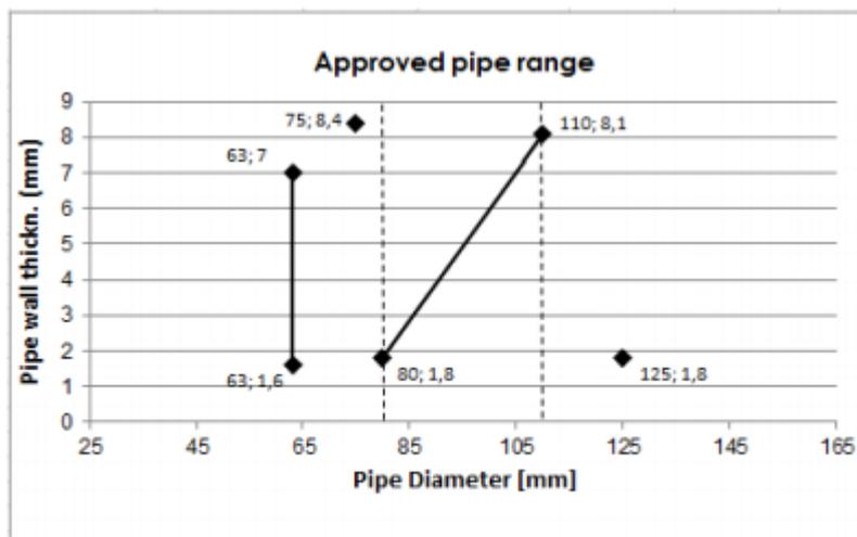
**2.2.4 PVC pipes acc. to EN 1452-2, EN 1329-1, EN 1453-1**
