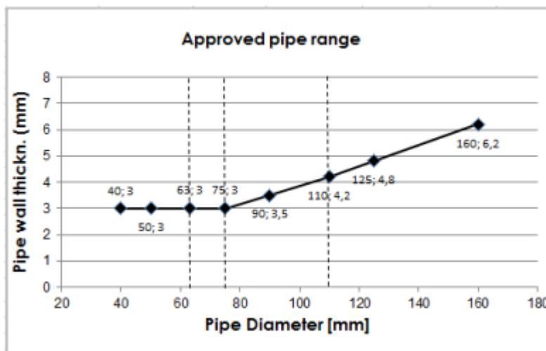
**2.2.1.2 PE pipes according to EN ISO 15494 and DIN 8074/8075**
