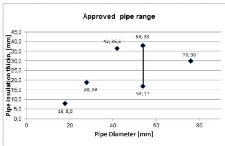
**2.2.10 Copper pipes including metal pipes,
