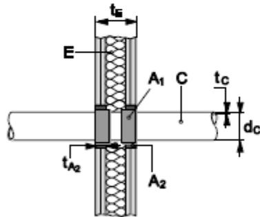
Application in a flexible wall (with Hilti Firestop Acrylic Sealant CFS-S ACR -  $A_2$ )
